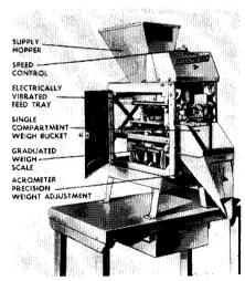
Elec-Tri-Pak weighing and filling machine manufactured by the Triangle Package Machinery Co. The weigher is of the semi-automatic type designed to fill dry material into any type container. Units are available to handle a weight range from 2 ounces to 5 pounds at a rate of up to 20 packages per minute PE2
